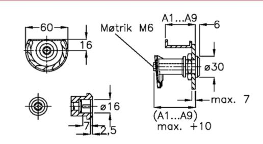
Door + frame thickness = 57-65 Measure type = A9
